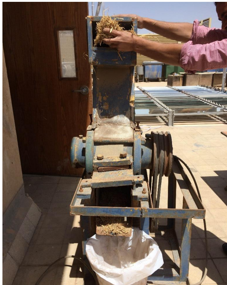
Figure 4 - Feeding large rice straws into the cutting machine to be cut into smaller straws
