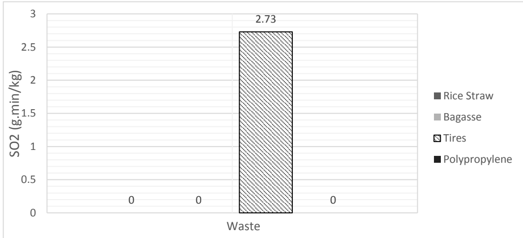
Figure 26 - SO 2 pollutant emission factors from burning rice straw, bagasse, tires, and polypropylene
